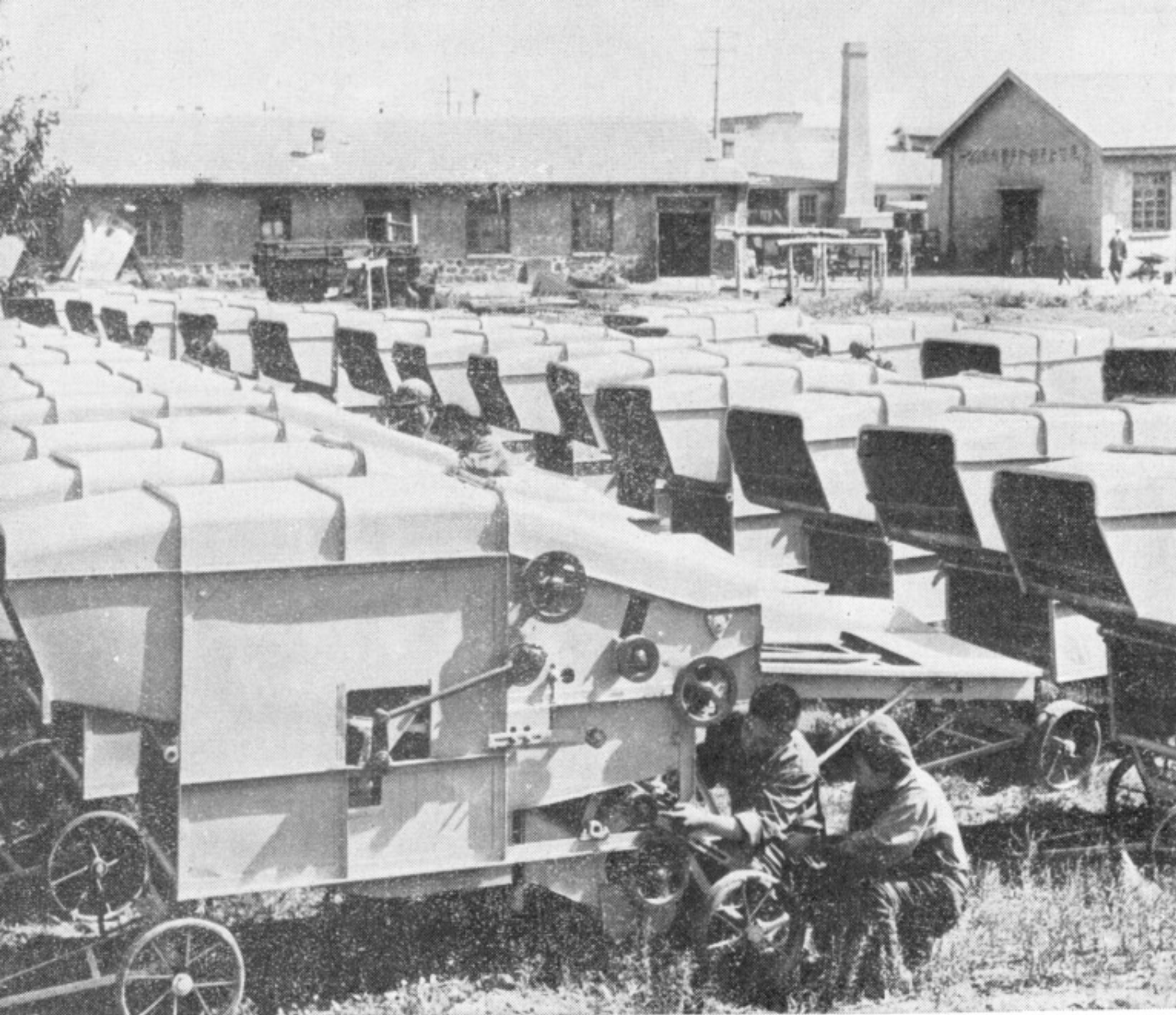
Final check of threshers — Changpei County Farm Implement Works in Hopei province.
